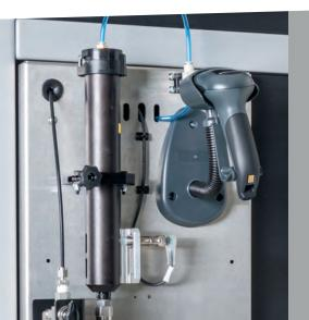
Consistently traceability via handheld bar code scanner and the material identification are logged!
